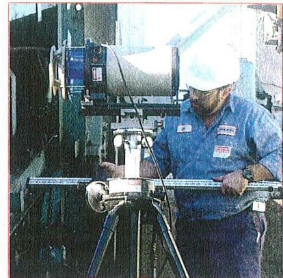
Figure 7. Taking measurements during a laser alignment survey.
