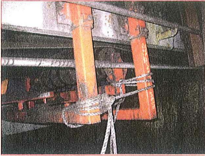
Figure 10. Conventional training idler tied off in one position, which is not solving the problem.
