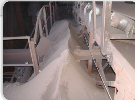
Conveyor Belt Mis-tracking, through the load causes material spillage on the walkways.
