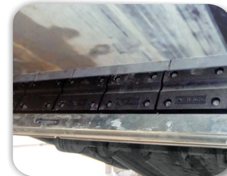
Toro secondary belt cleaner installed on the primary belt off the main crusher
