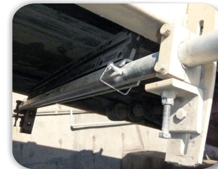
Toro secondary belt cleaner installed on the primary belt off the main crusher
