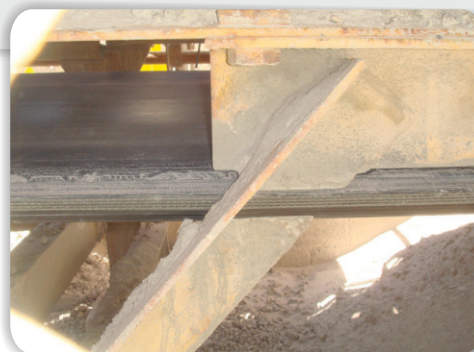
Mis-tracking , causing the conveyor belt to cut into the frame of the conveyor.
