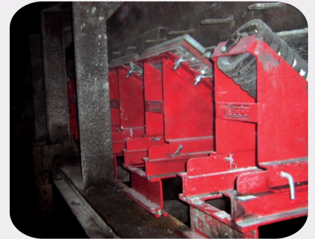
Modular Impact Beds installed on this coal handling conveyor at a major coal-fired power plant.
