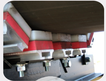
Modular Impact Beds installed on this coal handling conveyor at a major coal-fired power plant.
