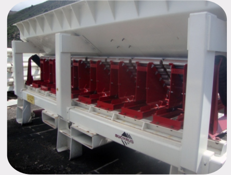
Modular Impact Bed installed on this tail section and about to be put into service at this western US underground coal mine.
