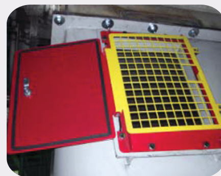
Door opened. Safety screen closed.
